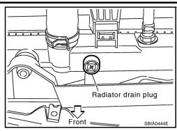
When draining all of engine coolant in the system, open water drain plugs on cylinder block. Refer to EM-246, "DISASSEMBLY".
