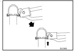
In areas where radiator plate pliers B cannot be used, use flat-blade screwdriver to bend the edge up.
