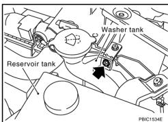
10. Rotate two radiator upper mount brackets 90 degrees in the direction as shown in the figure, and remove them.
