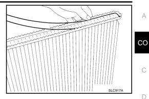
Caulk tank in numerical order as shown in the figure with radiator plate pliers A (SST).
