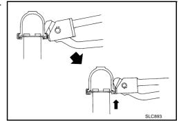
• In areas where the radiator plate pliers B cannot be used, use a screwdriver to bend the edge up.
