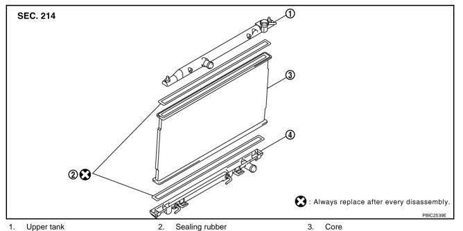
4. Lower tank (with A/T fluid cooler)
