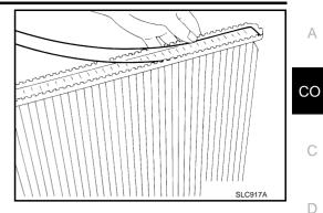
Caulk tank in numerical order as shown in the figure with the radiator plate pliers A [SST].
