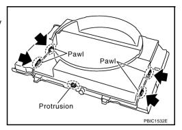
8. Lift up and remove radiator shroud.
